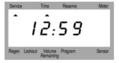
14. Flow Meter Equipped Valves Only: The Volume Remaining Display is the volume of water (In gallons) remaining prior to regeneration, including any reserve capacity. Without any water usage the Meter Arrow should be either off or on but not changing. Open a soft water tap. The Meter Arrow should begin flashing at a rate that varies with flow rate. Close the tap after 3-5 gallons of water flow.
