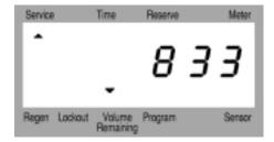
For Example: 833 Gallons Of Water Remaining (Valve in Service) Service Time Reserve Meter
